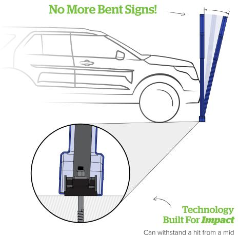
Can withstand a hit from a mid sized car traveling at 3 ½ mph
